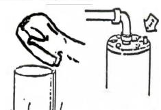
Connect a hose to a house spigot and run water directly into the well until chlorine odor is present in the water. Run the water this way for 15 minutes.
